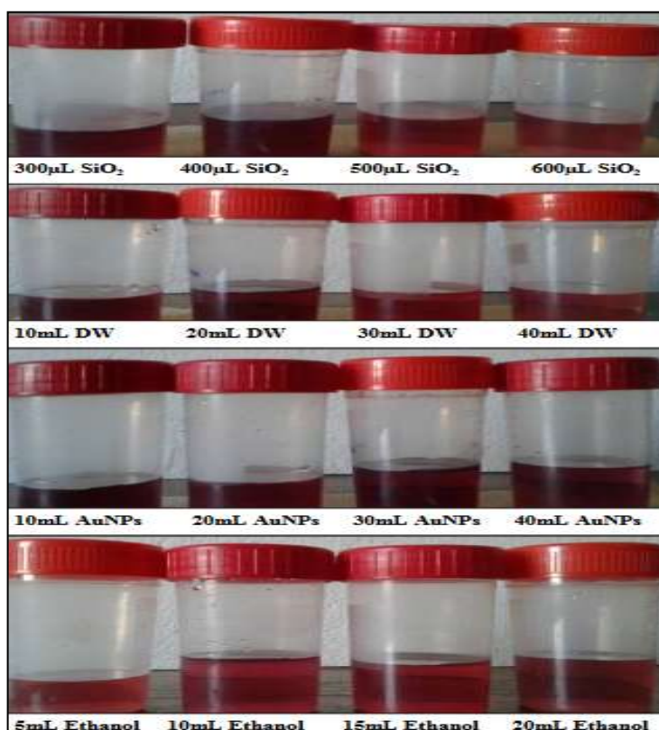
Fig 3.7: Coated gold nanoparticles under the effect parameters four \text{SiO}_2 content, deionized water volume, gold nanoparticles solution volume and ethanol volume.
